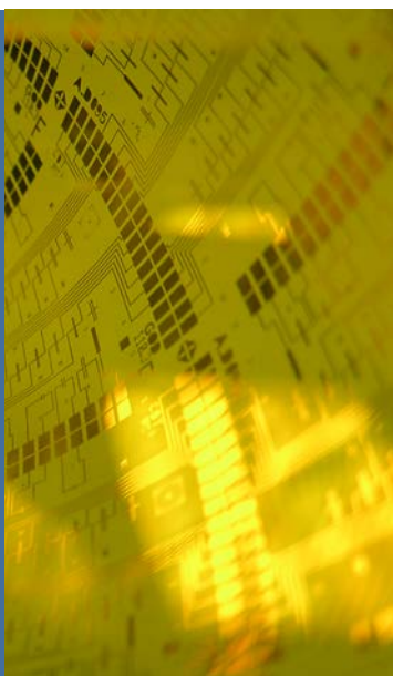
Lithographically defined electrodes on plastic film
